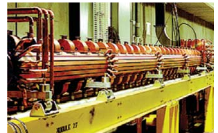
Figure 2. From 100 to 800 MeV The side-coupled linac accelerating structure (100 to 800 MeV) was invented by Los Alamos accelerator scientists during the design of LAMPF.
