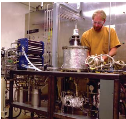
Figure 3. Equipment and Testing Brent Faulkner is pictured (photo taken around 1994) with the 10-kW electrochemical engine, a complete PEM fuel-cell power system, developed through a joint collaboration between the Laboratory and GM. The insulated components to the right are part of the methanol steam reformer that produced, on demand, hydrogen-rich gas from a liquid fuel. The two 5-kW PEM fuel cell stacks (made by Ballard) have blue endplates and can be seen at left. Additional equipment required to complete the power system is out of the photo frame.
